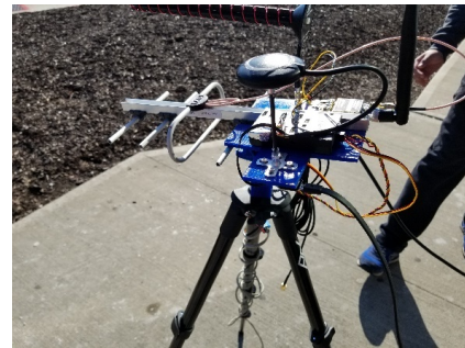
Figure VII. Preliminary Design of Antenna Tracker
